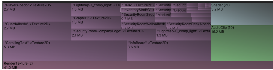
The Summary view also displays a Tree Map of memory usage for the time the snapshot was captured.
